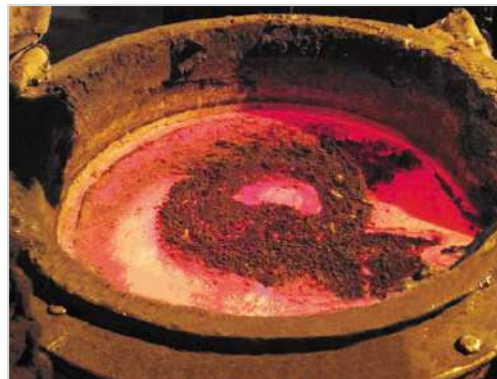
Figure 11: Photograph of extremely dry dross in transfer ladle after treatment with COVERAL MTS 1582.
