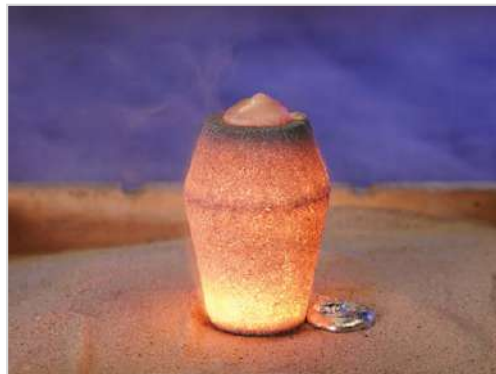
Figure 4. Constant burn-off of the FEEDEX NF1 feeder
