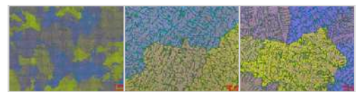
Figure 9a: Before treatment. Grain size d_m [ \mu\text{m} ] = 984
