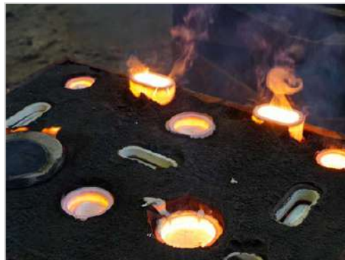
Figure 3: Clearly visible exothermic reaction of the FEEDEX NF1 riser
