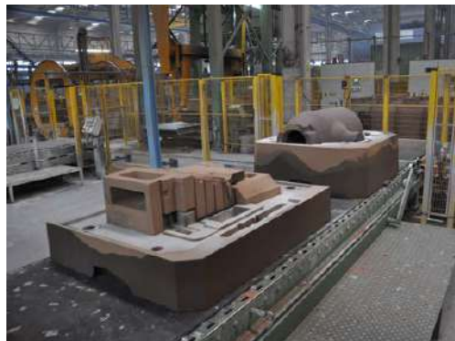
Fig. 3: Assembly of POLISET bonded moulds and POLITEC bonded cores
