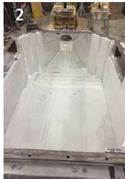
Figure 4: Insulating materials for floor and side walls
