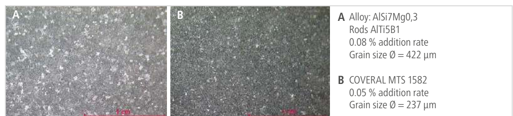
Figure 10: Comparison of TiB rods with Coveral MTS 1582: grain size
