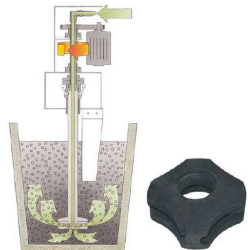
Figure 5: Effective degassing process using a Foseco Degassing Unit (left) and the patented impeller rotor (right)
