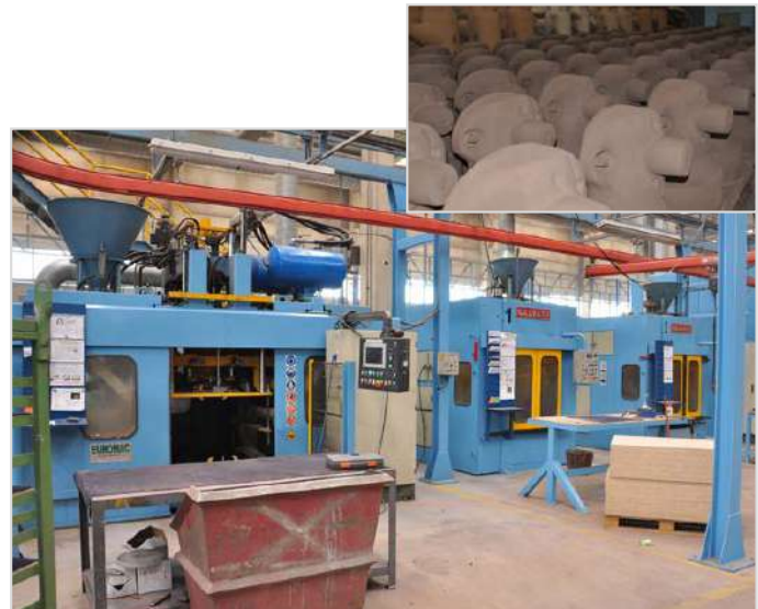
Fig. 2: Coreshop & cores coated with TENOTEC 7804A (inset) using the flow coating process
