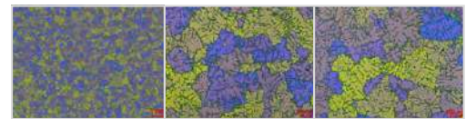
Figure 9b: After treatment. Grain size d_m [ \mu\text{m} ] = 206
